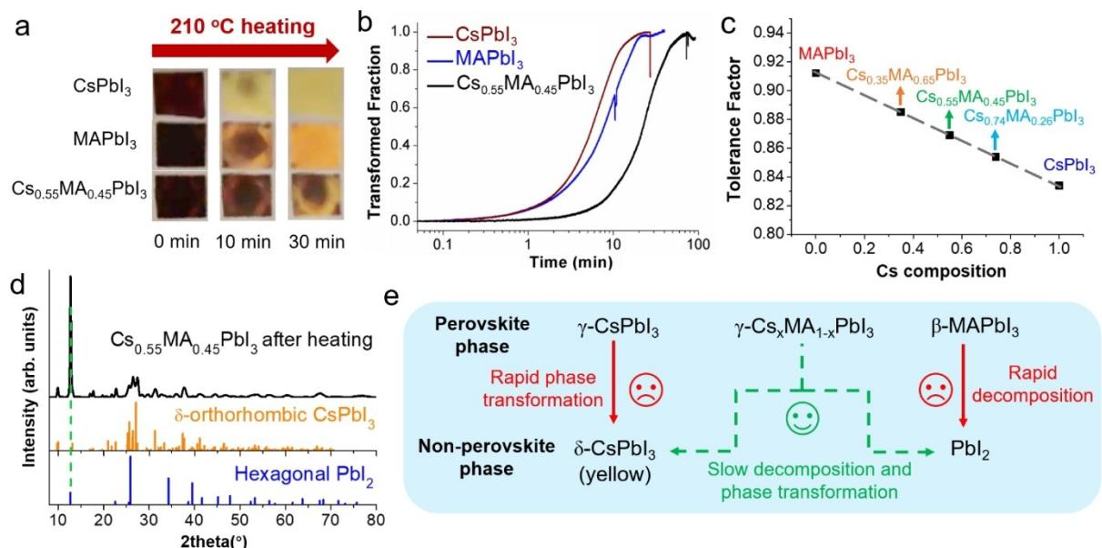
and MAPbI<sub>3</sub> nanocrystal films turned completely yellow in 20 min and 30–40 min respectively, while the Cs<sub>0.55</sub>MA<sub>0.45</sub>PbI<sub>3</sub> nanocrystals took ≈80 min to turn completely yellow.
