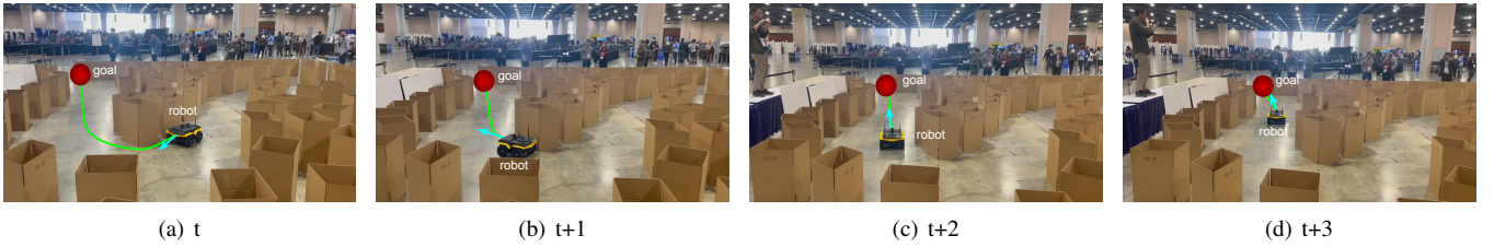
Fig. 15. Successful navigation behavior of the Jackal robot in the wide “S” shaped environment at different times.
