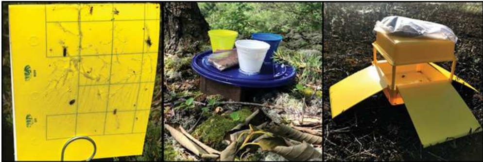
Figure 3. Sticky cards, bee bowls, and ramp traps (left to right) deployed at various field sites in the Southeastern Great Lakes Region in 2019.
