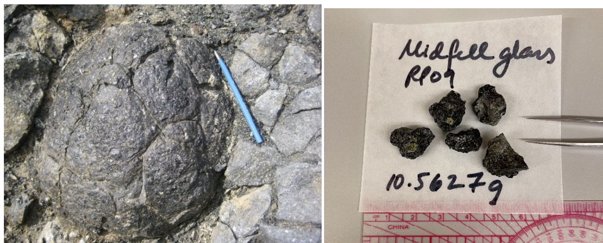
Figure S-1 Pillow basalt and MiðfellRP09 glass. (left) Vesicular, olivine phenocryst-rich basalt, glass was abundant (1/4" cold chisel for scale). (right) Five pieces of glass over 10 g in mass were analysed in a single crusher chamber.
