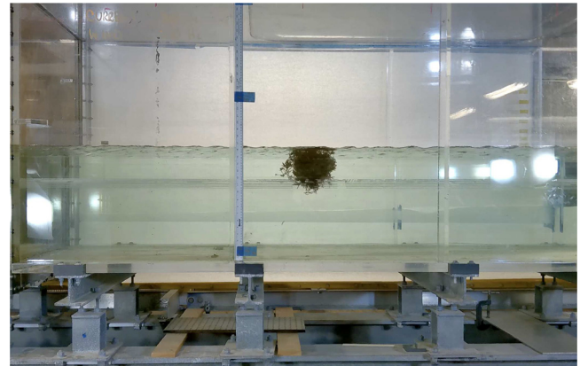
FIG. 1. Side view of the ASIST air–water stream flume where the Sargassum windage experiments were carried out. A Sargassum cluster, representative of those employed in the experiments, is shown floating at the water level. The clusters used were composed of clumps collected from a raft found in the Florida Current off the southeastern coast of the Florida Peninsula.
