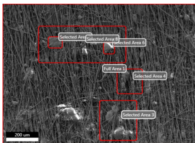
Fig. 6 EDAX Area Selection for Elemental Composition Analysis
