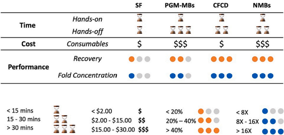
Fig. 6. Time, cost, and performance comparison of different concentration methods.
