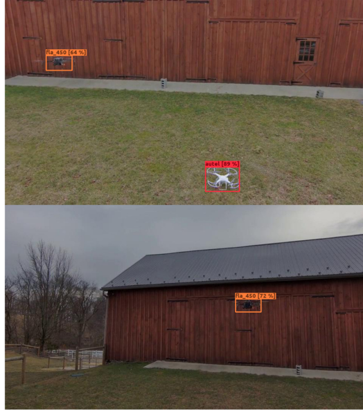
Fig. 17. Drone detection results by FPGA with bounding boxes on images from the multi-drone dataset.
