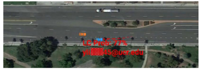
Fig. 6. Bird-eye's view application interface: digital twin of vehicles running on the edge server in real time.
