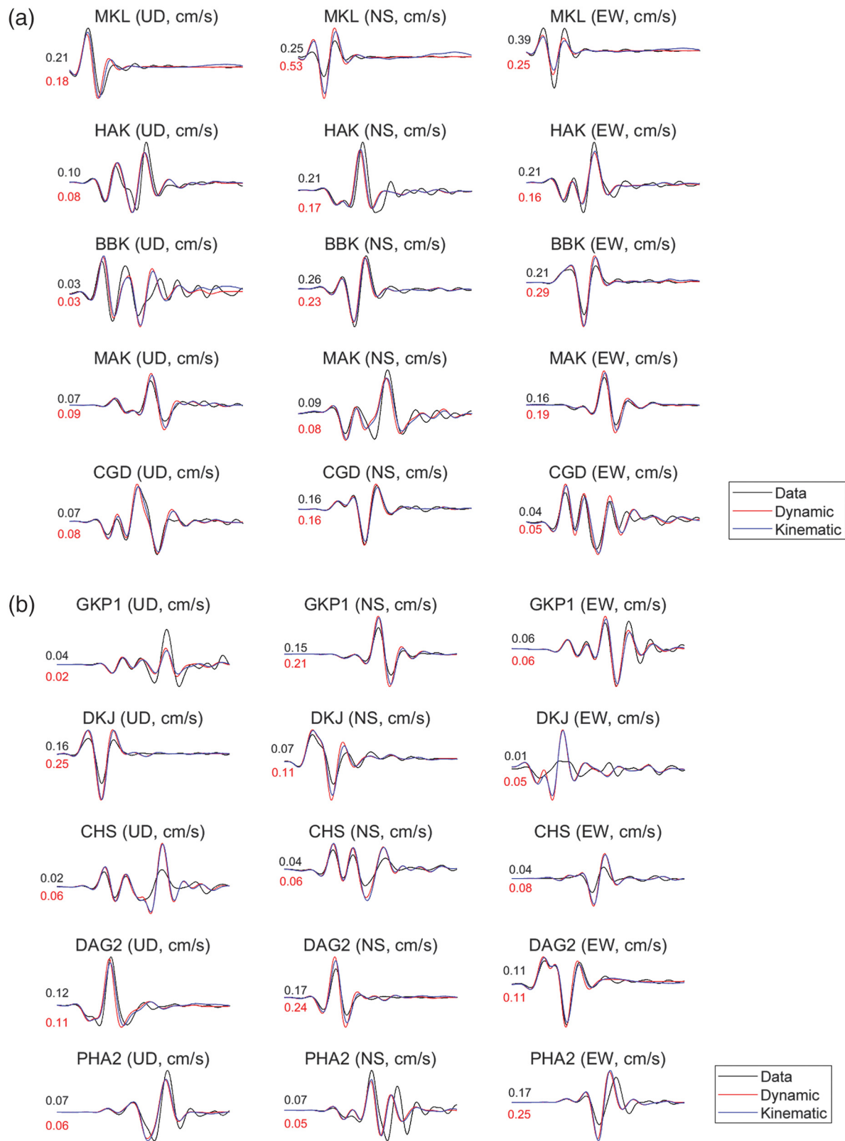
Figure 8. (a,b) Waveform comparison (0.05–0.3 Hz) for model II. (c,d) Waveform comparison (0.05–0.5 Hz) for model II. (e,f) Waveform comparison (0.05–1.0 Hz) for model II. (Continued)
