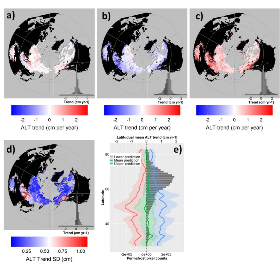
**Figure 5.** Spatial patterns of (a) mean, (b) lower prediction, (c) higher prediction, (d) standard deviation (SD), and (e) latitudinal summary of the ALT trend from 2003 to 2020 derived from the RF methods. Permafrost pixel counts used for latitude binning are denoted by gray bars, while the SD of trends for ensembles are represented by shaded colors in plot (e).
