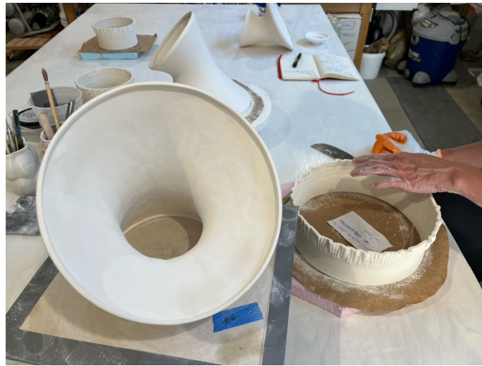
Figure 6: Left: Ceramic pieces at different stages: ring fresh off the 3d printer (front right), central module drying (back left), and central module waiting to be trimmed and sanded before bisque firing (front left).
