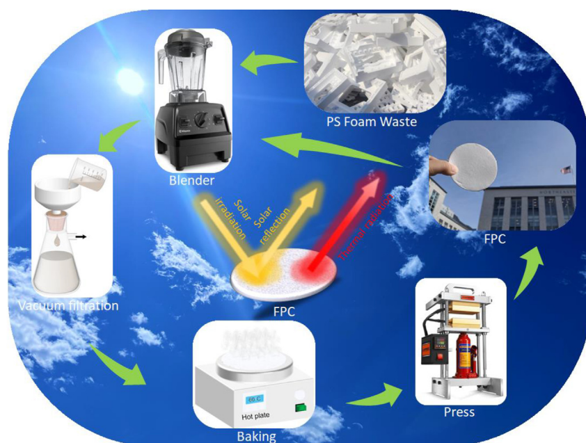
Fig. 1. Schematic illustrating the radiative cooling mechanism of the FPC and its closed-loop fabrication and recycling processes.
