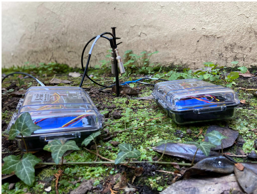
Fig. 17. SHT-30 sensors zip-tied to tent stake.
