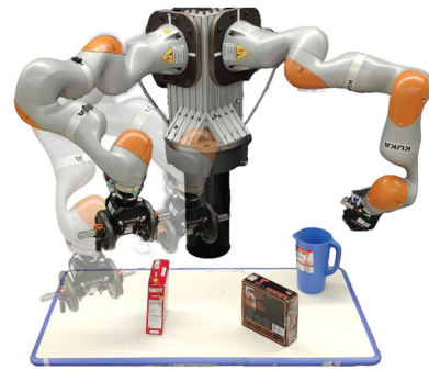
Fig. 1. 7-degree-of-freedom manipulator carrying a weight in a cluttered environment with uncertain tracking control.
