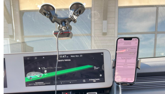
Fig. 3: Data collection setup mounted on vehicle windshield with Racebox GPS receiver and data logging on the dashboard-mounted smartphone.
