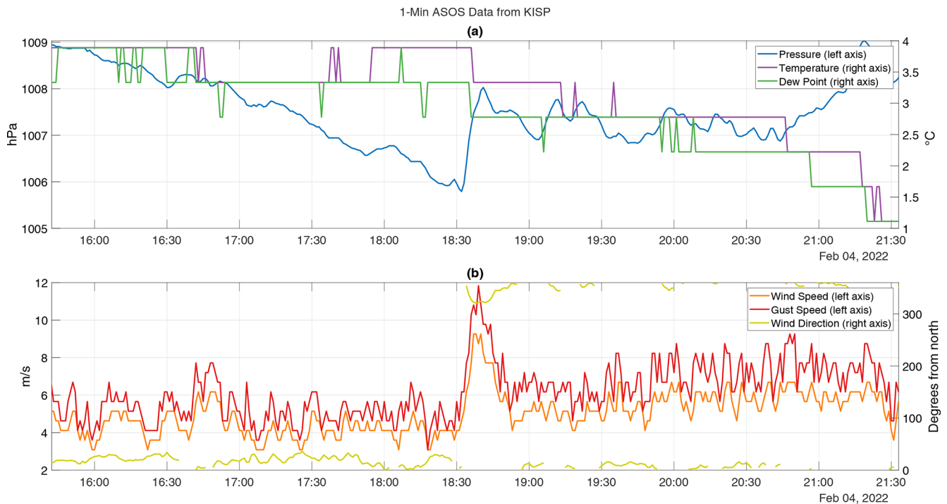
Figure 13. Time series of 1 min ASOS data from Islip, NY (KISP), on 4 February 2022. (a) Temperature (purple), dew point (red), and pressure (blue). (b) Wind speed (orange), wind gust speed (red), and wind direction in degrees clockwise from northerly (yellow). Wind direction is not plotted when it changes by more than 180^\circ in consecutive observations (e.g., when crossing 0 or 360^\circ ) or when the wind speed is below 1.5 \text{ m s}^{-1} . All times are UTC.
