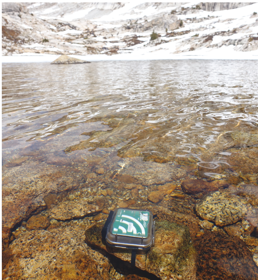
Figure 1: AudioMoth acoustic recorder deployed underwater at the study site.
