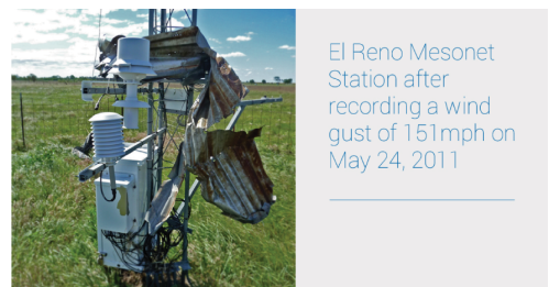
(b) A destroyed Oklahoma Mesonet station following a severe wind gust
