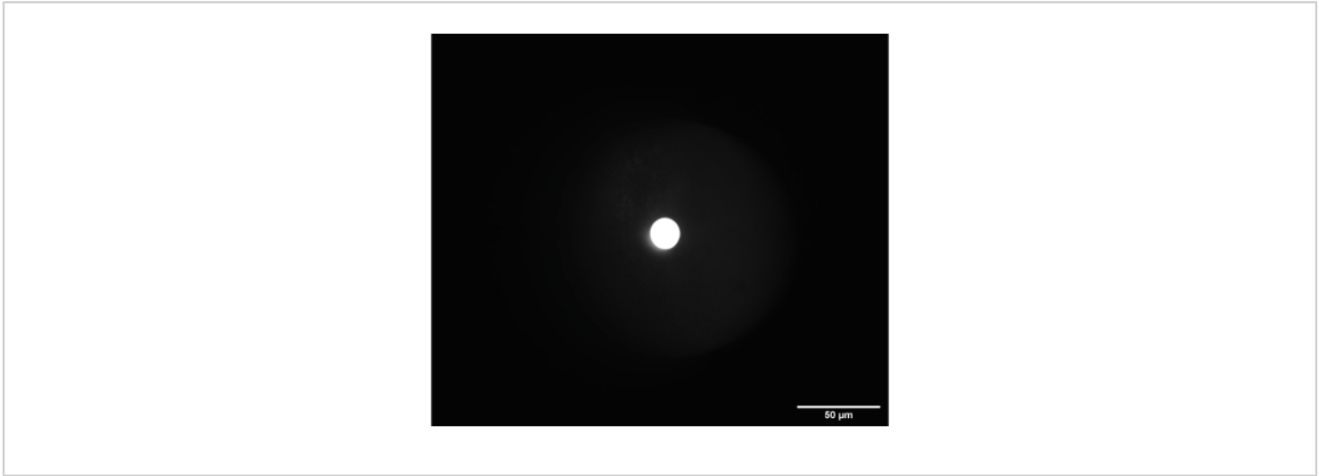
Figure 6: On-camera image of the correctly focused frosted glass alignment disk. The disk was placed at the intermediate plane between SL2 and TL2. Scale bar = 50 μm. Abbreviations: SL2 = scan lens; TL2 = tube lens. Please click here to view a larger version of this figure.
