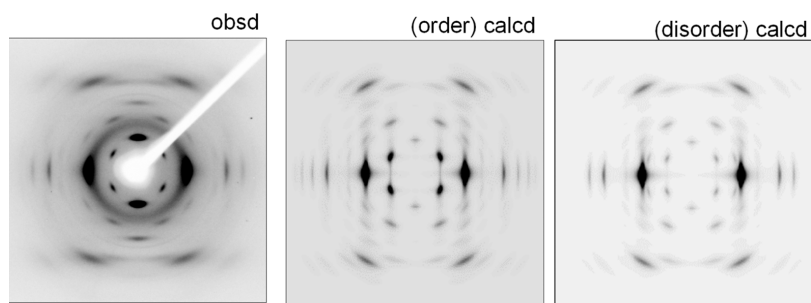
Figure 6. Comparison of the observed 2D WAXD pattern of it-PPMA sample with those calculated for the ordered and disordered models (refer to Figures 2 and 5). The incident X-ray beam is Mo K\alpha with a wavelength of 0.7107 Å.
