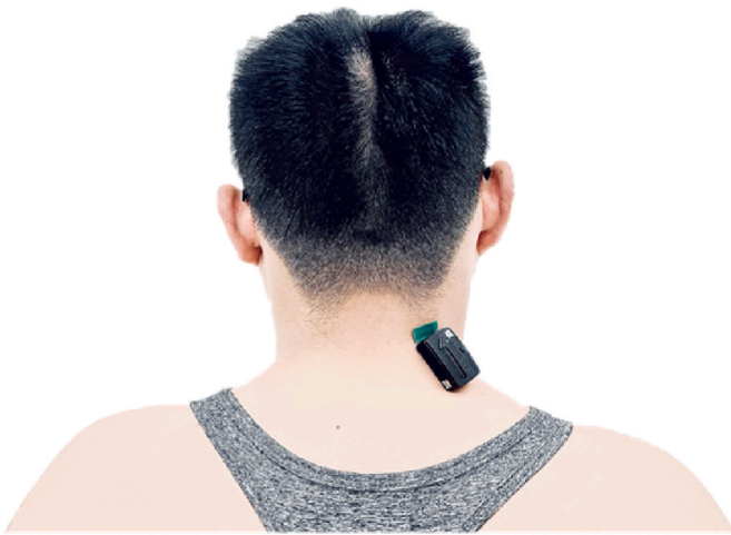
Fig. 7. The EMG sensor at upper right trapezius muscle.
