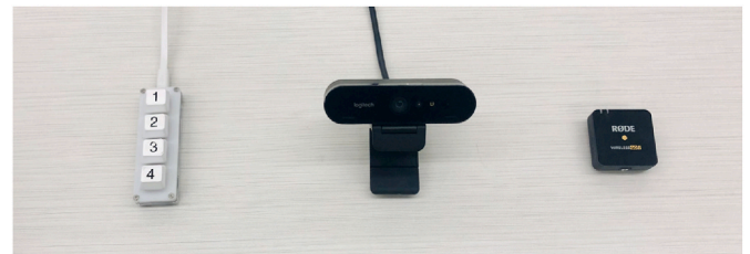
Fig. 3. Devices used to interact with the co-robot (from left to right): extended keyboard, webcam, and wireless microphone.
