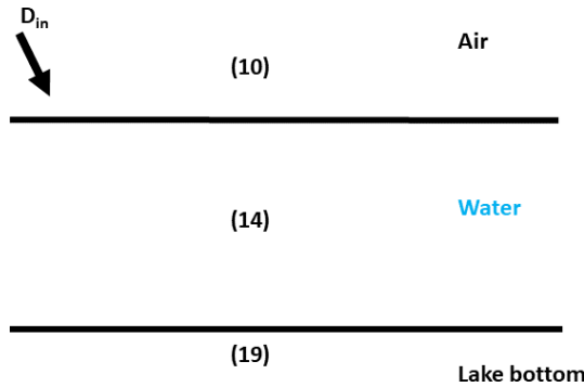
Figure 4. A schematic of the no-lake-ice stage of the lake-refreezing module. D_{in} represents the depth of meltwater contribution (in metres) to the lake from its corresponding hydrological catchment in every time step. Equations (10) and (19) are solved at the air–water and water–lake-bottom interfaces, respectively. Equation (14) is solved for the water in the lake. We assume that the lake bottom is an impermeable surface, i.e. ice or saturated firm or snow.
