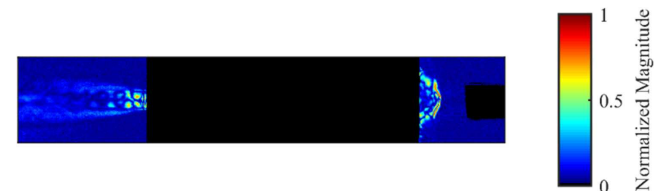
Fig. 9 Contour mapping of the relative intensity of the 20 kHz peak from Schlieren images.
