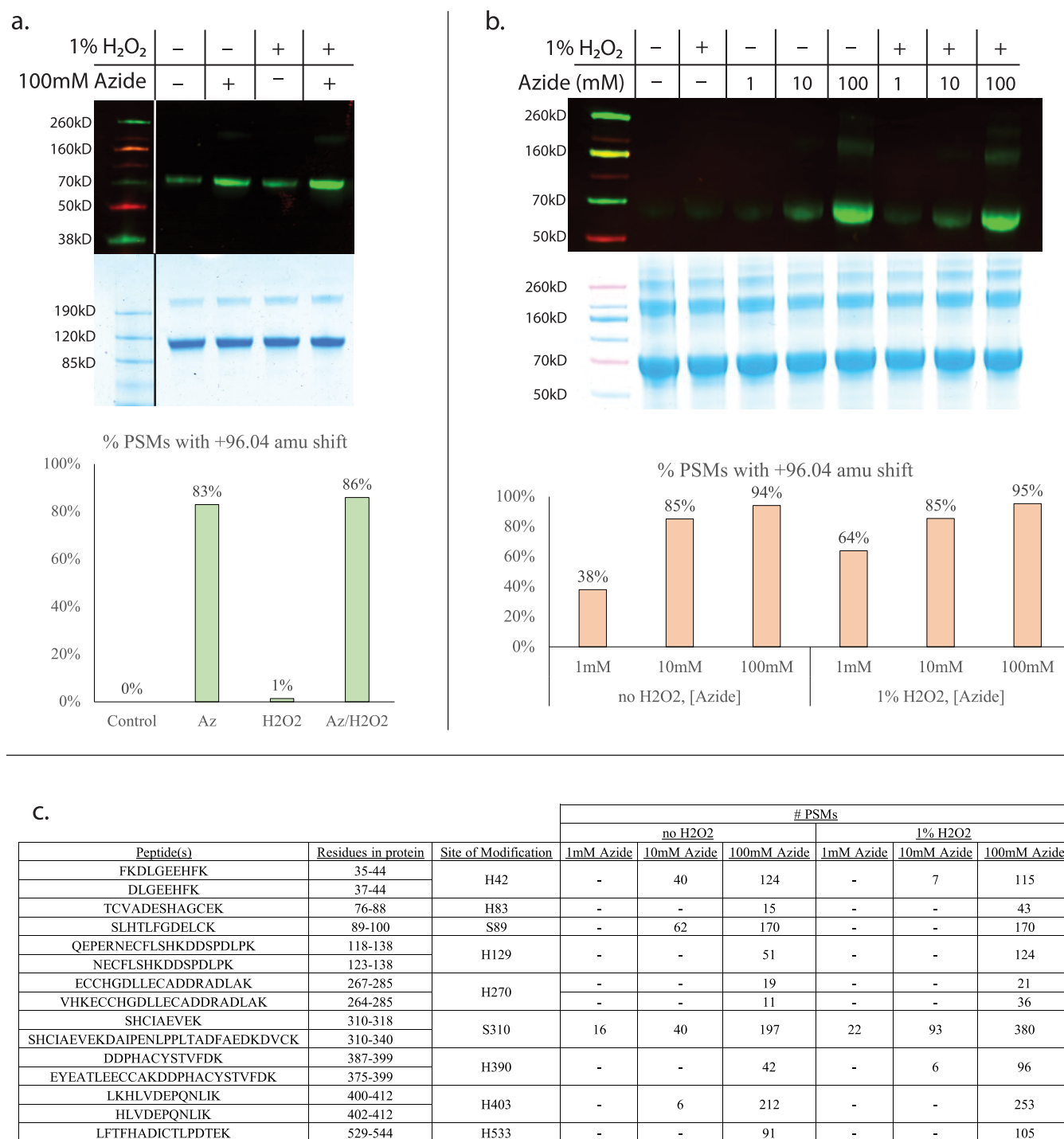
Figure 3. BSA is azidylated in an azide-dependent fashion. (a) Top: Streptavidin blot using a copper and alkyne-based conjugation system visualized by fluorescently-labeled streptavidin. Middle: Coomassie-stained polyacrylamide gel. Ladders and lanes are from separate regions of the same gels and not vertically shifted (gray and black lines, respectively). Bottom: Though fluorescence is observed in lanes without peroxide and azide, no modification is observed via mass spectrometry. (b) BSA azidylation is azide dose-responsive, and at lower concentrations, peroxide causes increased azidylation over azide alone. Top: Streptavidin blot. Middle: Coomassie-stained polyacrylamide gel. Bottom: Similar levels of azidylation are observed via mass spectrometry with 100 mM azide \pm peroxide, lower levels with 10 mM azide and added peroxide, and higher levels with 1 mM azide and added peroxide. (c) In BSA, azide dose-dependent azidylation occurs mainly on histidine and serine.
