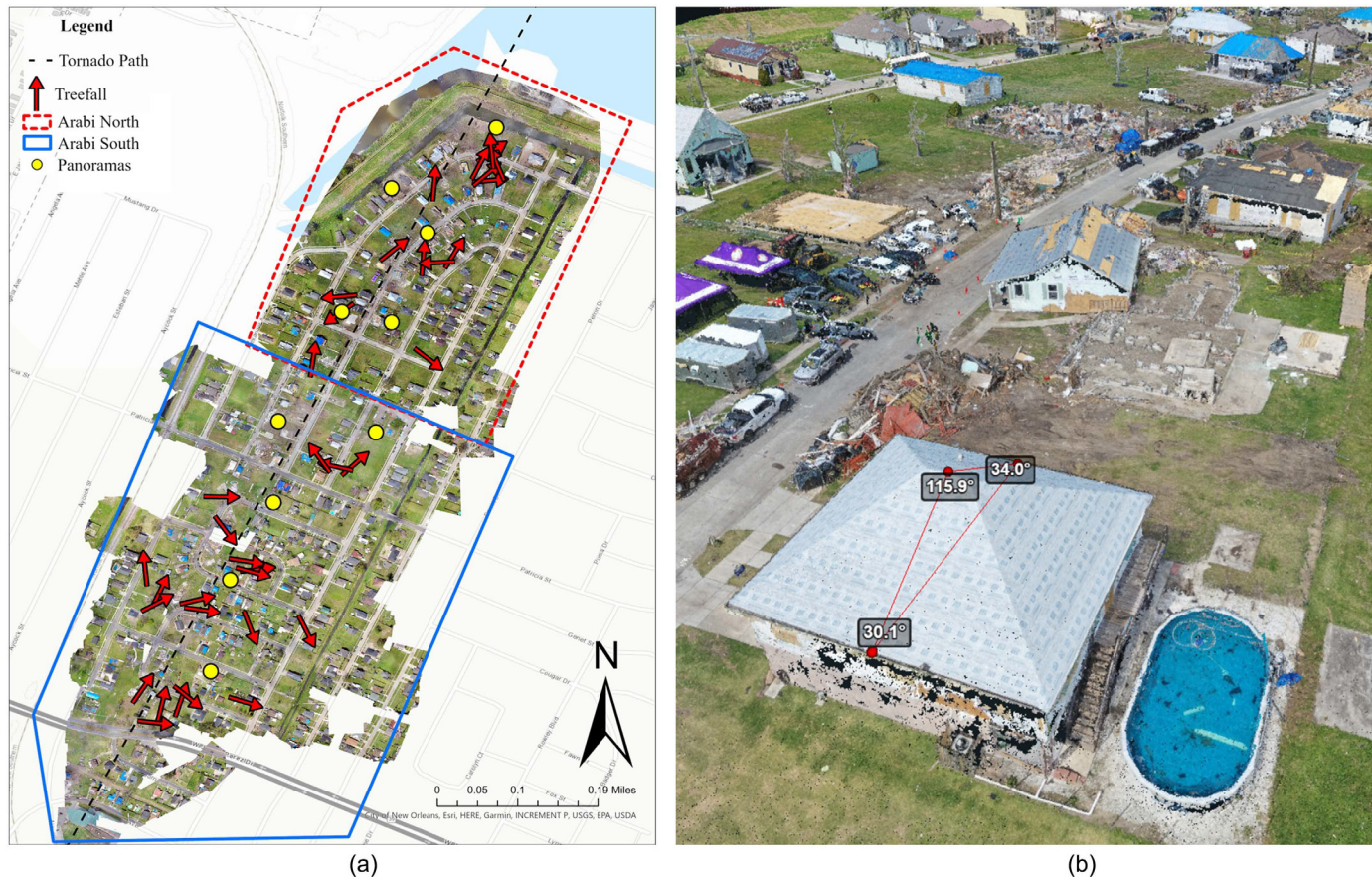
Fig. 3. UAS flights (a) preplanned flight area of the north (dashed line) and south (solid line) Arabi and locations of the additional panoramas (filled circles) (sources: Esri, City of New Orleans, HERE, Garmin, INCREMENT P, USGS, EPA, USDA); and (b) processed point cloud from the Arabi North flight with the ability to measure dimensions and other physical parameters (image by authors).
