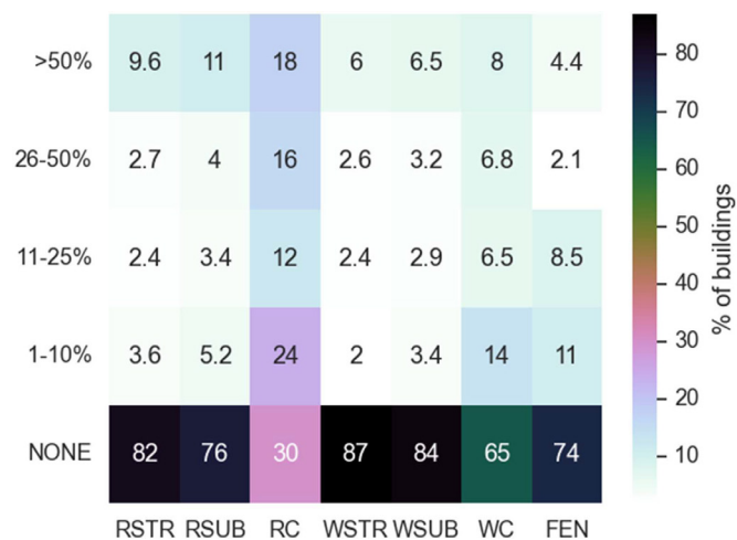
Fig. 11. Frequency (%) of component damage for damages states of none, 1%–10%, 11%–25%, 26%–50%, and greater than 50%. RSTR = roof structure; RSUB = roof substrate; RC = roof cover; WSTR = wall structure; WSUB = wall substrate; WC = wall cover; and FEN = fenestration.
