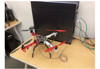
Figure 5: Drone HITL Validation.
