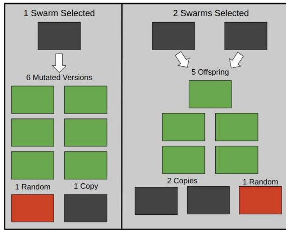
Fig. 9. A diagram showing how the next generation of controllers is produced in our implementation of Swarm Chemistry. The process differs depending on the number of controllers the user selects.
