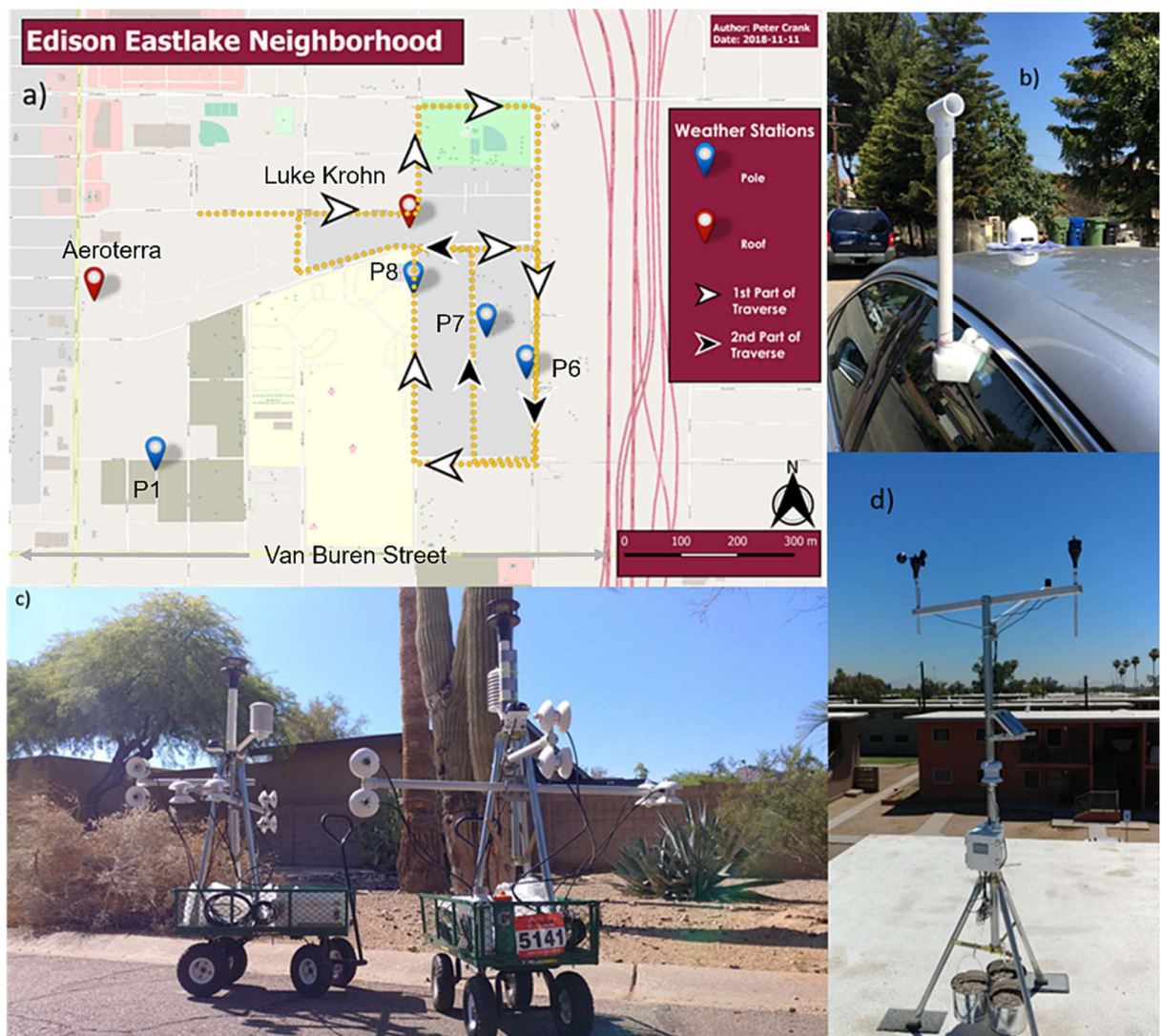
Fig. 2. Map of the weather stations, the mobile traverses, and the instruments used. A) shows the route for the traverses and the location of fixed weather stations (P7 was lost/disappeared during data collection), b) is the car traverse thermocouple, c) shows the two MaRTy carts (Middel and Krayenhoff, 2019), and d) shows a fixed weather station. The traverses in this neighborhood only used one cart.
