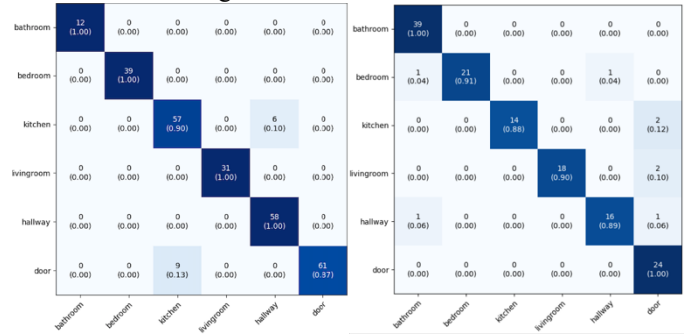
Fig. 8. The confusion matrix of location recognition. Robot view(Left), watch view(Right).
