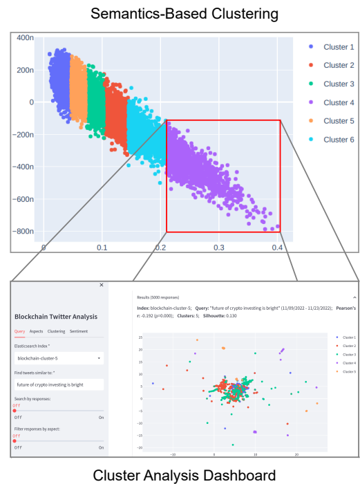
Figure 2: Pipeline of the two-stage topic clustering process. 1) The BERT embeddings are used to form clusters of the entire dataset using K-means. 2) Each cluster is then examined manually via a web dashboard for further analysis.
