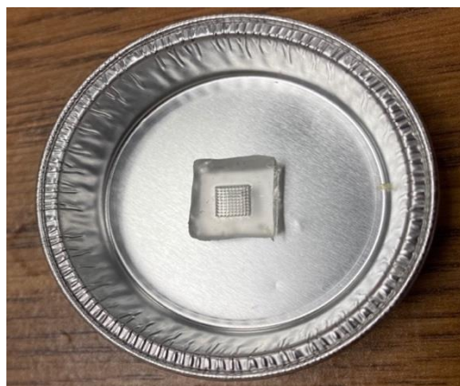
Figure 2. PDMS female microneedle array mold.
