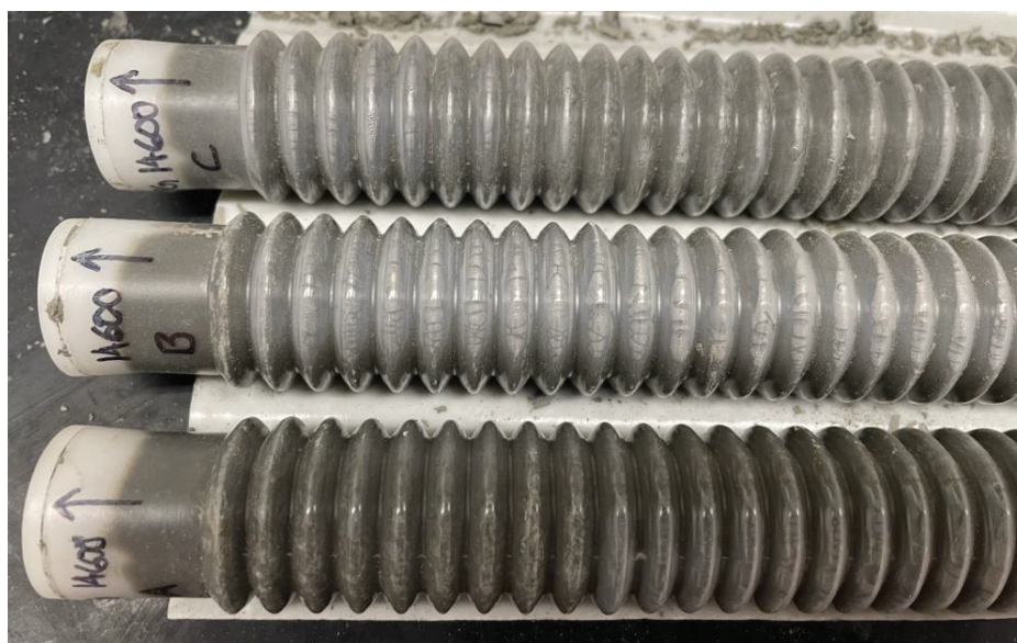
Figure 1. Corrugated tubes filled with fresh paste, used to measure the autogenous shrinkage.
