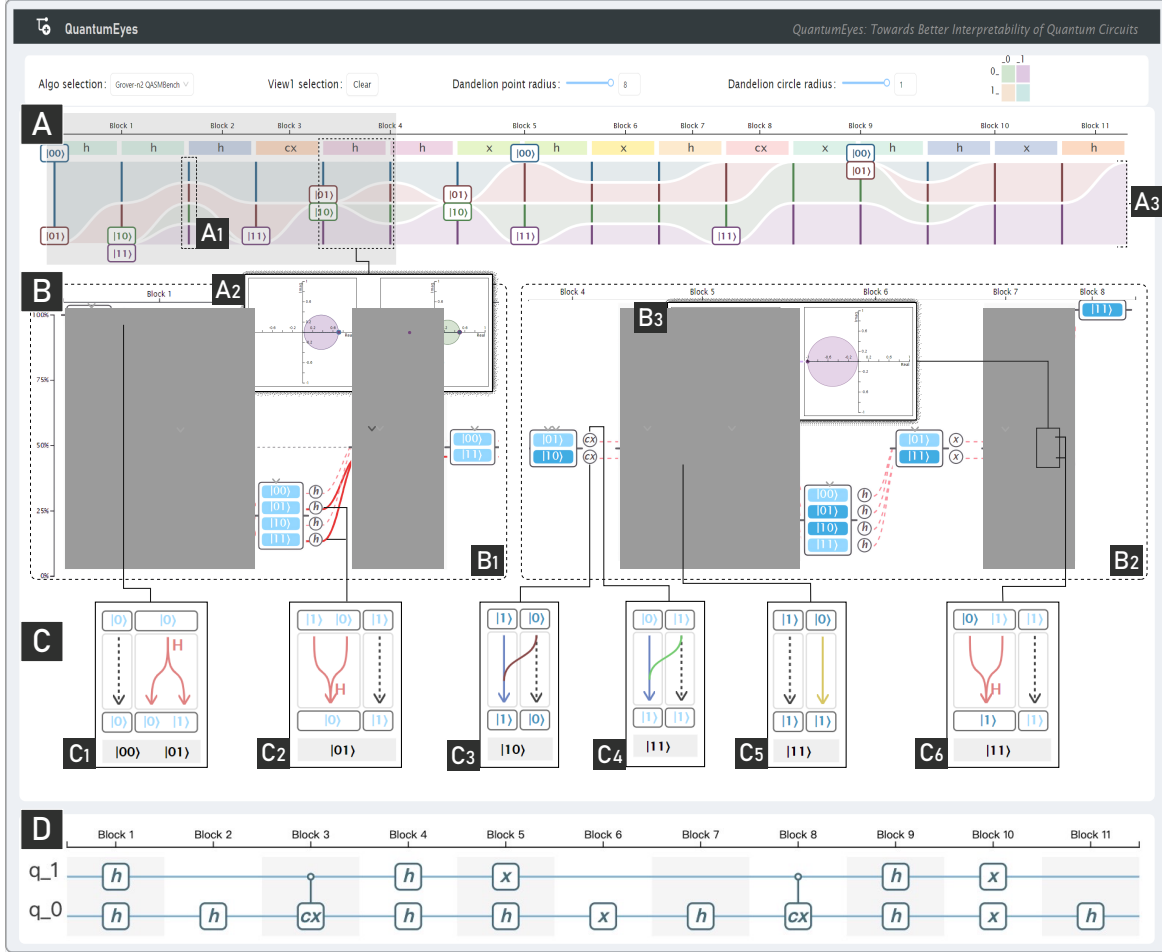
Fig. 1: The visualization system QuantumEyes enhances the interpretability of quantum circuits through the global analysis (A-C) to explain the operations of quantum gates and local analysis ( A_2 and B_3 ) to reveal the implicit reasoning of basis state's measured probability. Probability Summary View (A) shows the overview of a quantum circuit regarding the measured probability. State Evolution View (B) supports the in-depth analysis of the basis states across each step. Gate Explanation View (C) explains the effects of quantum gates via the transformation of qubit states. State Comparison View ( A_2 and B_3 ) with the geometrical visualization dandelion chart enables users to better understand the measured probability regarding amplitudes. The original quantum circuit (D) is given for a better comparison of QuantumEyes and quantum circuit diagrams.
