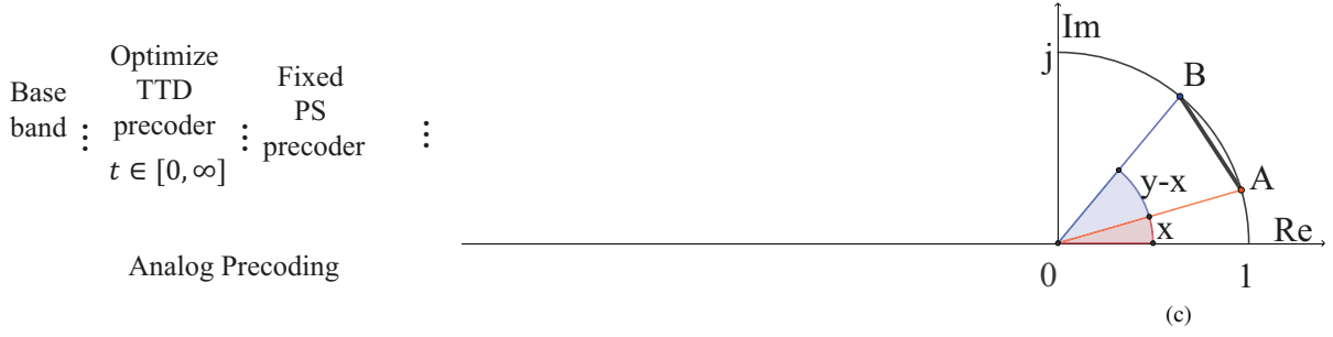
Fig. 2. (a) Conceptual illustration of the prior methods for beam squint compensation [10], [12], [13]. (b) The proposed method of this work. (c) Conceptual illustration showing the relationship between the distance of two points on the unit modulus circle (the segment AB) and their relative phase difference (the arc corresponding to y - x )
