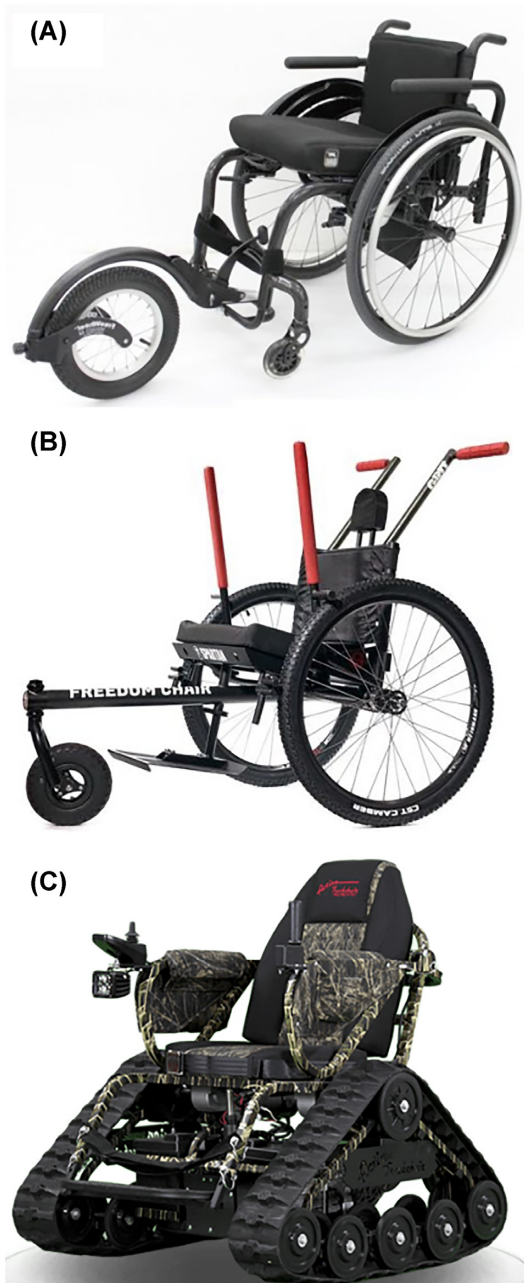
Fig. 1 Examples of (A) a FreeWheel wheelchair attachment (Northpole, United States), which clips to an existing manual wheelchair to improve off-roading ability, (B) a GRIT Freedom Chair (GRIT, Medford MA, United States), a manual all-terrain wheelchair, and (C) an Action Trackchair (Action Trackchair, Marshall MN, United States), a powered all-terrain wheelchair. Photos copyright to FreeWheel, GRIT, and Action Trackchair, respectively.
