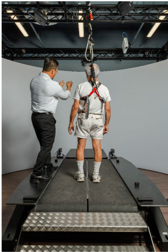
FIGURE 3 GRAIL system with dualbelt instrumented treadmill.
