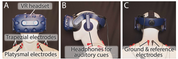
Fig. 1. Equipment setup for controlling the virtual reality ARM. (A) Front view showing the VR headset which was equipped with eye-tracking and a gyroscope. Pairs of sEMG electrodes were placed along the bellies of the left and right upper trapezius and platysma muscles to record muscle activity. (B) Side view showing the headphones used to give auditory cues during the experiments. (C) Back view showing the locations of the sEMG ground and reference electrodes.
