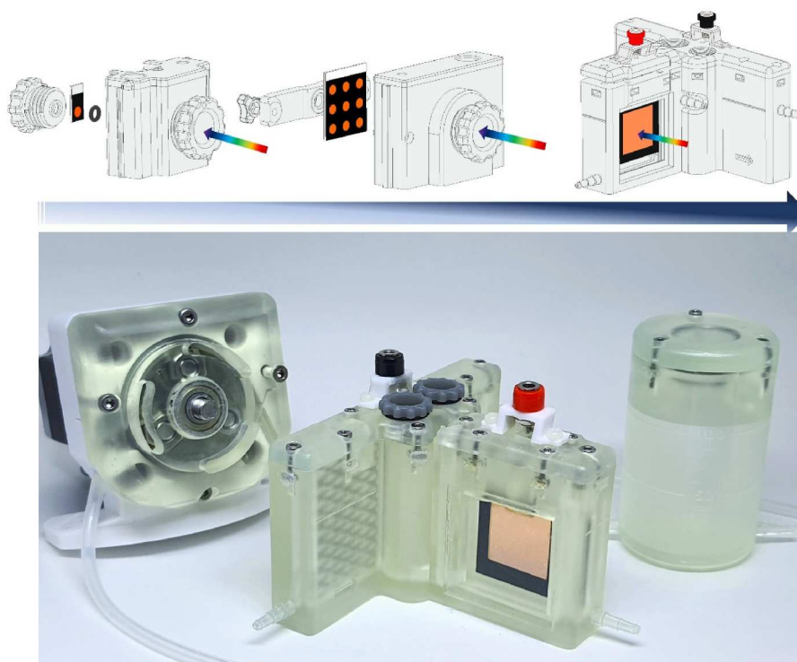
Fig. 2. (Top) From left to right, the representative image of 3D printed reactors with different dimensions and quartz windows for photoelectrochemical (PEC) evaluation under continuous electrolyte flow. (Bottom) Image illustrating the 3D printed PEC cell for larger electrode analysis ( >15 \text{ cm}^2 ). After printing using the Clear resin, the employed condition and post-cured was carried out with 1.25 \text{ mW/cm}^2 of 405 nm LED light for 60min at 60^\circ \text{C} . Although the seller did not provide details about resin formulation, the printed/post-cure system must be able to resist aggressive environments such as NaOH at high concentrations.
