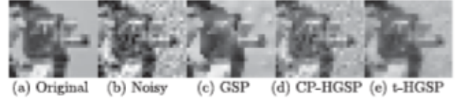
Fig. 13. (a) Zoom of the original Cameraman image. The image was contaminated with (b) Gaussian noise and denoised with (c) GSP, (d) CP-HGSP and (e) the proposed t-HGSP framework.
