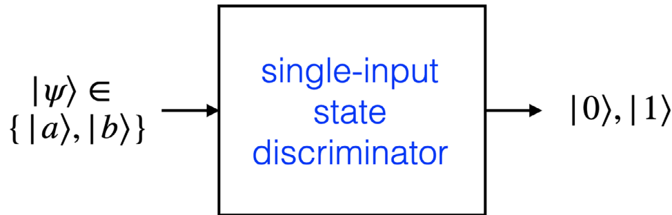
Figure 2. State discrimination channel. Here \langle a|b\rangle \neq 0 but \langle 0|1\rangle = 0 , so the channel must be nonlinear. Note that the output is always a basis state, |0\rangle or |1\rangle , simplifying readout.
