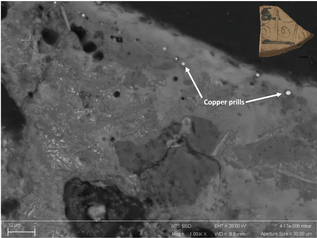
Fig. 12. Backscattered electron (BSE) image of the heterogeneous lead-alkali glaze on sample K254. The circular white inclusions visible near the surface of the glaze are metallic copper prills.
