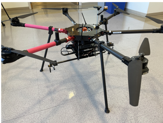
Fig. 1: PN with USRP B210 and 4 stub antennas, mounted on a UAV
