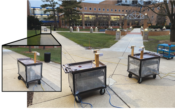
Fig. 2. Experimental setup. Nodes 0 and 1 are on the left and right, respectively, and the target oscilloscope cart is shown in the inset.
