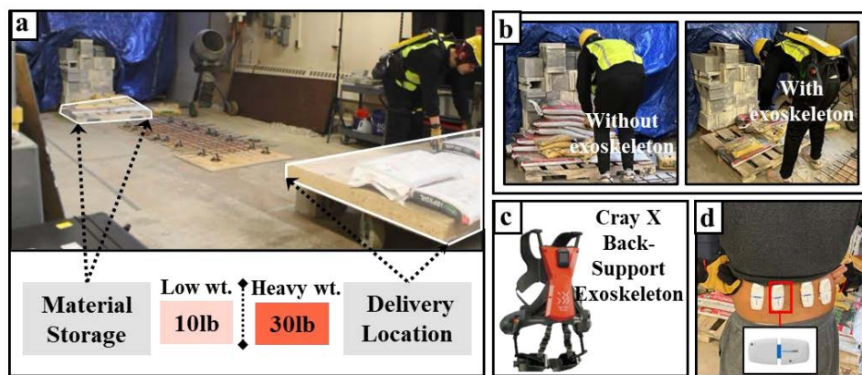
Figure 2. Case Study Illustration: a) Material handling task setup; b) Task with and without exoskeleton c) Active back-support exoskeleton; d) Placement of EMG sensor
