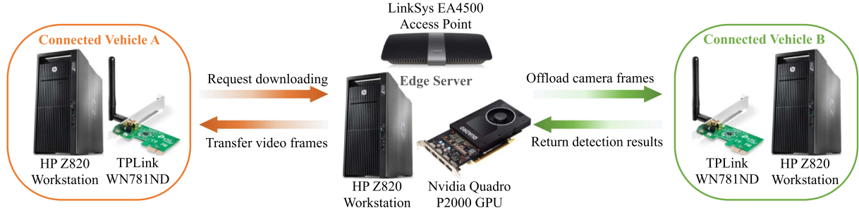
Fig. 1. Overview of the testbed implementation for our preliminary experiments. It consists of three components: an edge server and two connected vehicles. The edge server is built upon an HP Z820 workstation equipped with a NVIDIA QUADRO P2000 GPU and a LINKSYS EA4500 AP which is directly connected to the workstation through an Ethernet cable. To eliminate the impact of different wireless network cards on the experiment results, two emulated connected vehicles are deployed with the same TPLINK-WN781ND wireless network cards. Connected vehicle A downloads entertainment video frames from the edge server, while connected vehicle B offloads its camera image frames to the edge server for conducting object detection.
