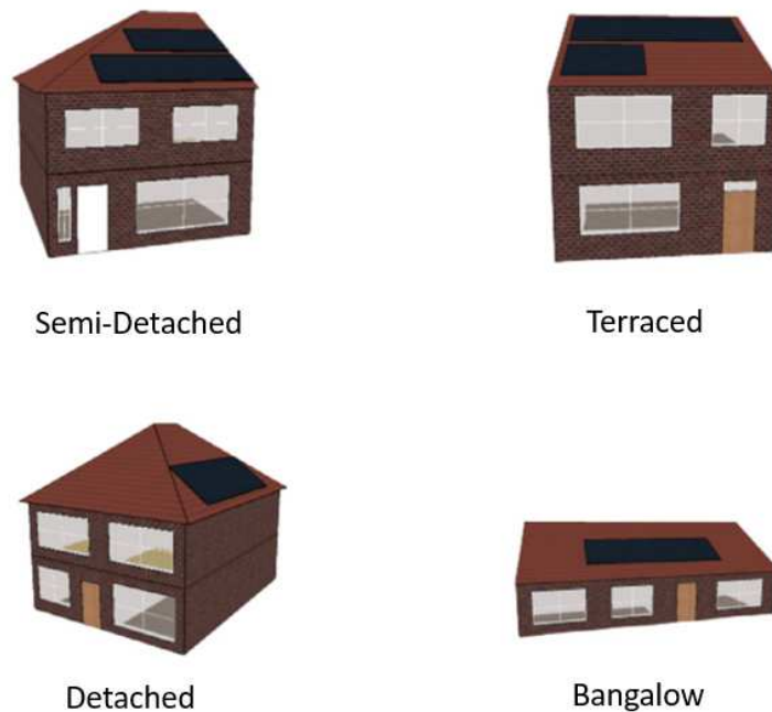
Figure 2 The geometric model of Irish residential building archetypes for energy parametric simulation for Dublin City [1]
