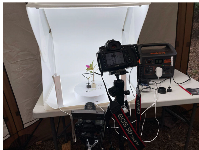
FIGURE 1 The battery-powered Foldio set-up with our two cameras on tripods set at different heights and a supplementary LED light on the hot shoe of the lower camera inside our pop-up work shelter. The scene demonstrates the use of an alligator clip to support the positioning of a branch in the center of the turntable, with the end of the branch anchored in a water-containing Eppendorf tube surrounded by modeling clay. The two 10-cm scale bars are attached to the turntable with double-sided tape.
