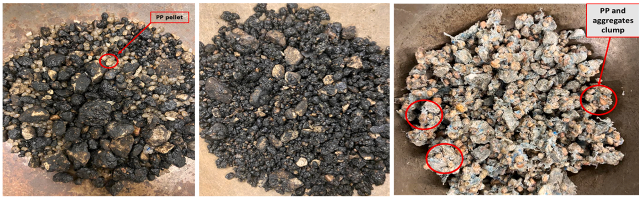
Fig. 5. PP mixed with RAP at 156° C (left), RAP at 180° C (center), and virgin aggregates at 180° C (right).
