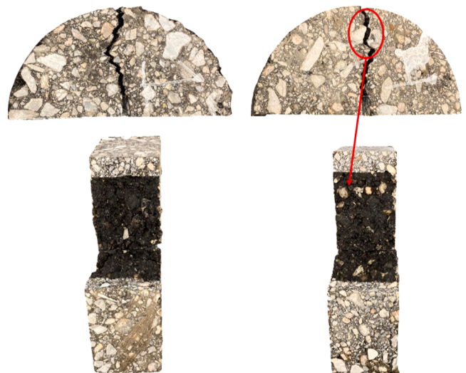
Fig. 8. Development of fracture path outside and inside of the test specimen left- SPR-MB-PP2 & right- SPR-MB-PP3.
